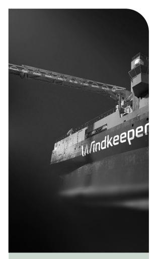
WindKeeper is an innovative Service Operation Vessel (SOV) based on Small Water Area Twin Hull (SWATH) methodology and design
